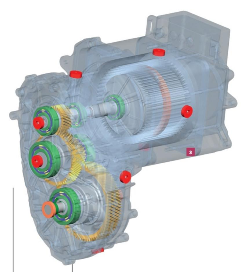
2. Drivetrain casing in MASTA, implemented as one finite element mechanical model of the entire casing around the gearbox and motor
