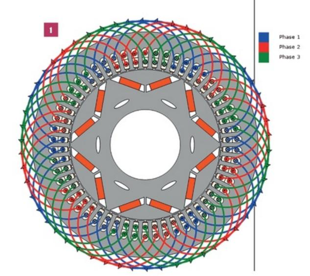
Even highly complex winding arrangements can be accommodated by MASTA 12 within the machine – and numerically, in charts and tables of quantities such as voltages, flux linkages and torque. The finite element model can also generate D- and Q-axis flux maps, used to quickly calculate torque-speed curves, efficiency maps and current and phase angles required to generate a desired torque at a specified speed.
