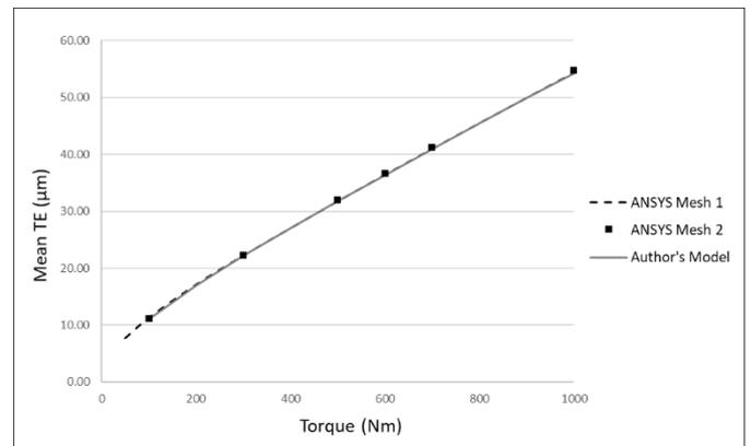
Fig. 7 Comparison of Author's model and ANSYS. Mean Transmission Error (μm) against load
