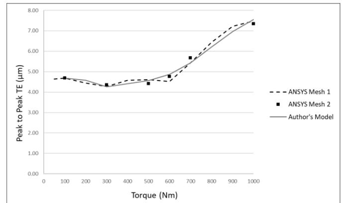
Fig. 6 Comparison of Author's model and ANSYS. Peak-Peak Transmission Error (μm) against load.
