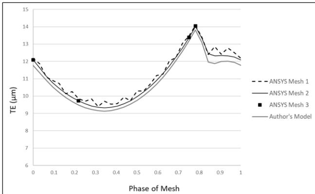
Fig. 5 ANSYS convergence study at 100 Nm Torque on drive flank. Transmission Error (μm)
