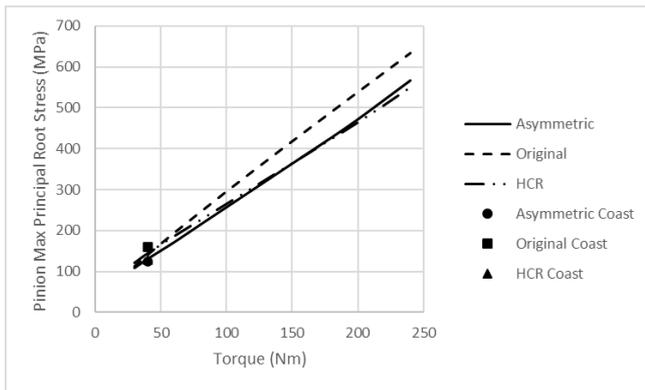
Fig. 13 Comparison of Pinion Max Principal Root Stress (MPa) against load
