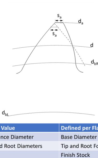
Fig. 2 Asymmetric Gear Geometry
