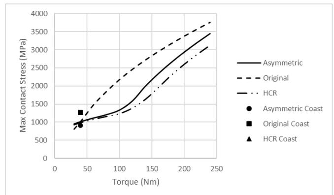
Fig. 12 Comparison of Maximum Contact Stress (MPa) against load
