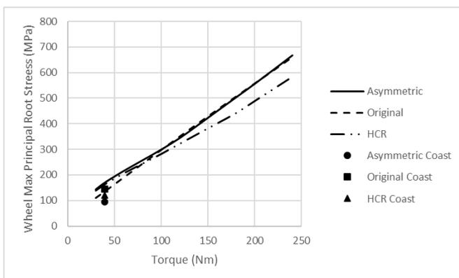
Fig. 14 Comparison of Wheel Max Principal Root Stress (MPa) against load
