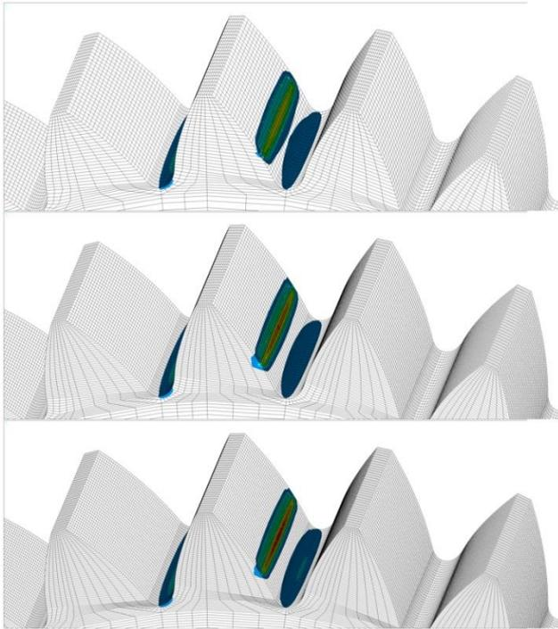
Fig. 4 ANSYS meshes; from top to bottom – Mesh 1, Mesh 2, Mesh 3
