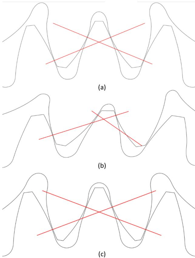
Fig. 10 Comparison of tooth shapes (a) Original, (b) Asymmetric and (c) HCR
