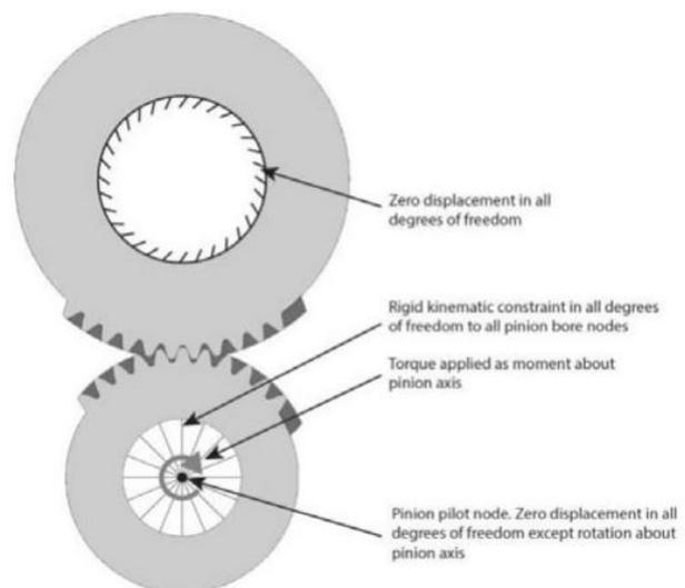
Fig. 3 Schematic diagram showing the displacement and force boundary conditions applied to the FE model
