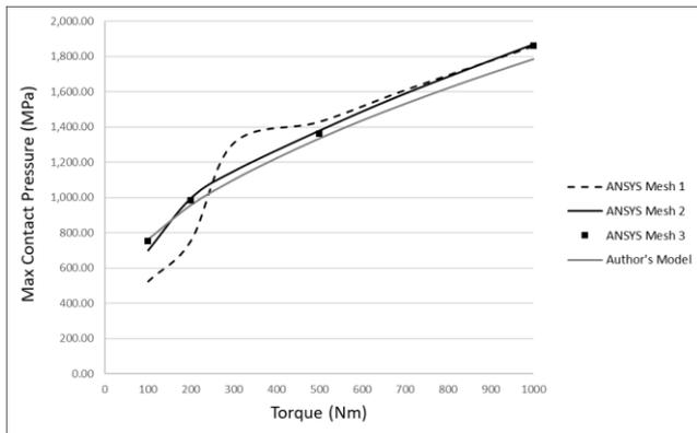
Fig. 9 Comparison of Author's model and ANSYS. Maximum Contact Stress (MPa) against load
