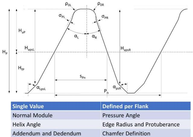
Fig. 1 Asymmetric Rack Geometry
