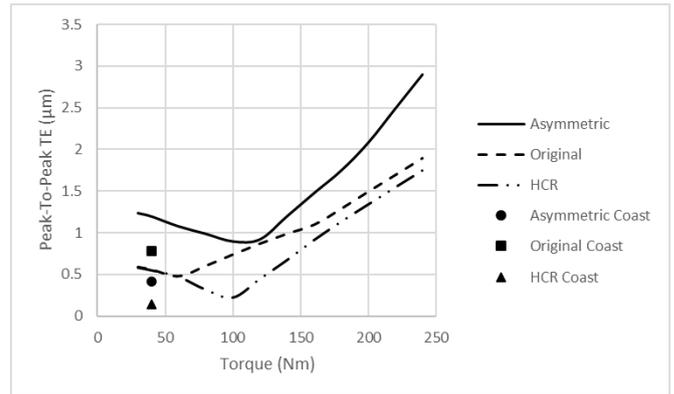
Fig. 11 Comparison of Peak-to-Peak Transmission Error ( $\mu\text{m}$ ) against load
