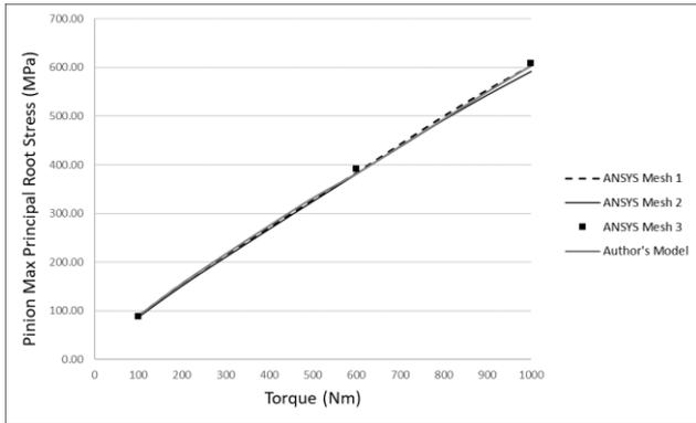
Fig. 8 Comparison of Author's model and ANSYS. Pinion Max Principal Root Stress (MPa) against load
