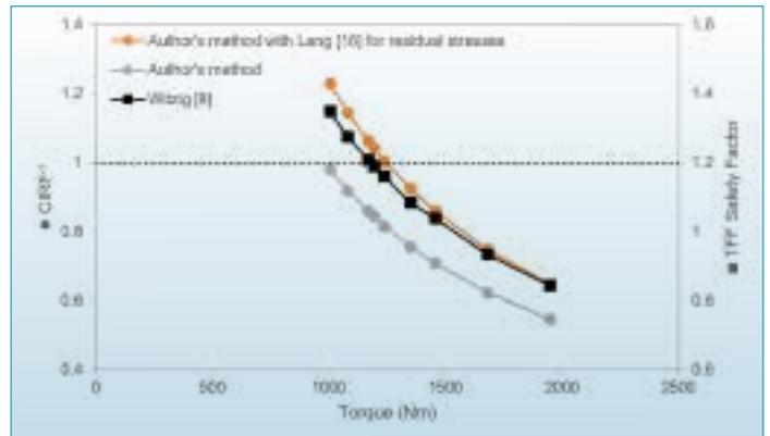
Figure 5 Comparison of calculated CIRF<sup>-1</sup> and Witzig's method for 67/69 Spur Gear. It should be noted that y-axis of the TFF safety factor is shifted to give comparable results (i.e. threshold value for CIRF<sup>-1</sup> is expected to be 1 and for TFF safety factor is 1.2 [8]). Adapted from Al, et al. [14]
