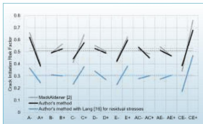
Figure 3 Comparison of the effects of individual factors and their interactions on CIRF response for author's method, author's method with Lang<sup>[16]</sup> for residual stresses, and MackAldener's FE calculations. The dotted lines represent the mean response from each method. As shown in Al et al.<sup>[12]</sup>
