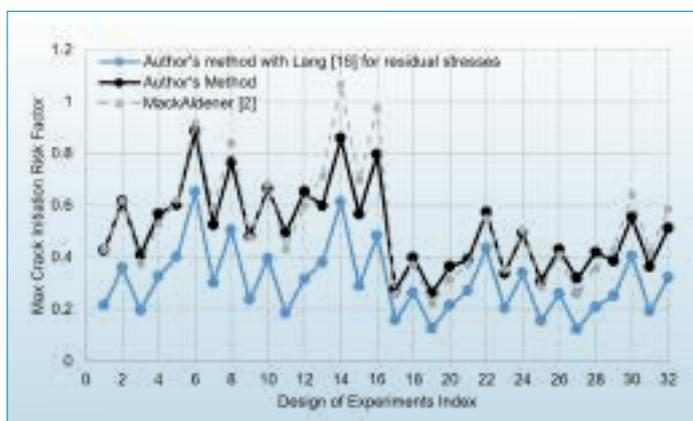
Figure 2 Comparison of the calculated Maximum CIRF's using the author's method, author's method with Lang<sup>[16]</sup> for residual stresses, and MackAldener's finite element calculations. Index values have been determined by first sorting according to factor (A through E) then sorting the values of each factor in ascending order. As shown in Al et al.<sup>[12]</sup>
