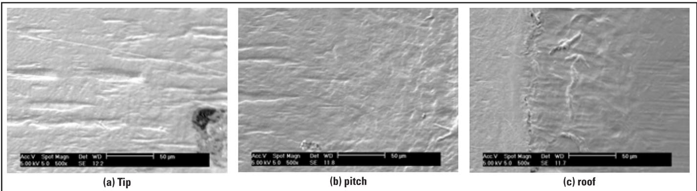
Figure 7 PA gear tooth SEM results.
