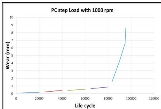
**Figure 2 Experimental results for polycarbonate gears.**
