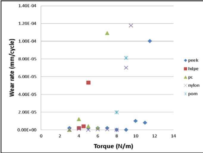
Figure 5 Wear rate against load for the same five polymer gear pairs.
