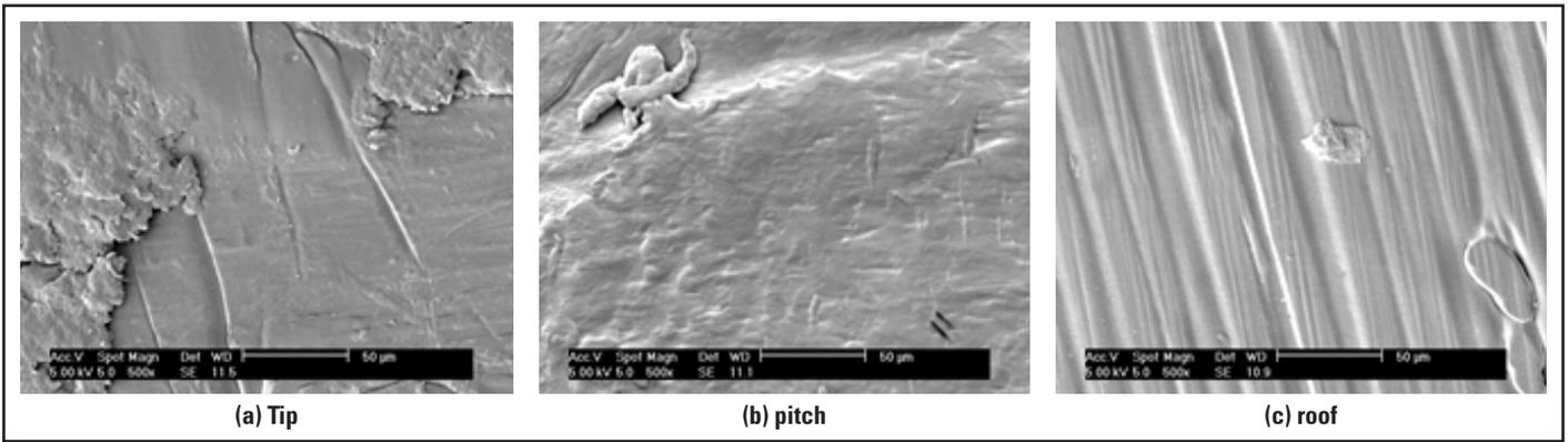
Figure 6 PEEK gear tooth SEM results.
