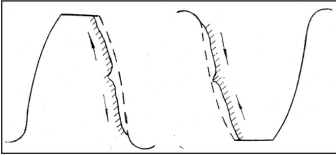
Figure 4 Gear surface wear (Ref. 2).
